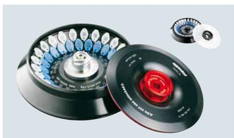
**Rotor for 48 × 1.5/2.0 mL tubes** spins up to 18,210 × *g*/12,700 rpm (FA-45-48-11\*/\*\*\*; Order no. 5427 754.008). Also available with basic plastic lid (F-45-48-11\*\*\*; Order no. 5427 755.004).
