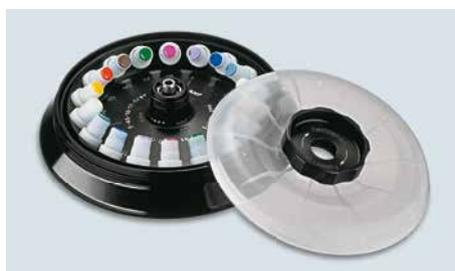
**18-place rotor for CryoVial® and HPLC tubes.** Speed up to 8,324 × *g*/8,900 rpm (F-45-18-17-Cryo; Order no. 5427 705.007 incl. cryo adapters).
