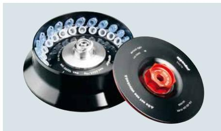
**Eppendorf Kit rotor** for 24 × spin columns and 1.5/2.0 mL tubes. Designed with an extra high rim to support open tube lids during centrifugation. Spins at max. 19,090 × *g*/13,200 rpm (FA-45-24-11-Kit\*; Order no. 5427 752.005).
