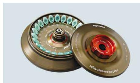
**High-speed rotor for 24 × 1.5/2.0 mL tubes** spins up to 30,130 × *g*/17,500 rpm for fast separation results. (FA-45-24-11-HS\*\*/\*\*; Order no. 5427 710.000).
