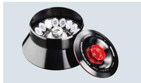
**Rotor for 16 × 5.0 mL Eppendorf Tubes** for speed up to 21,190 × *g*/14,200 rpm (FA-45-16-17\*/\*\*\*\*; Order no. 5427 750.002). Adapters for smaller tubes available: > 1.5/2.0 mL, pk/4 (Order no. 5820 768.002) > Cryogenic tubes, pk/4 (Order no. 5820 769.009)
